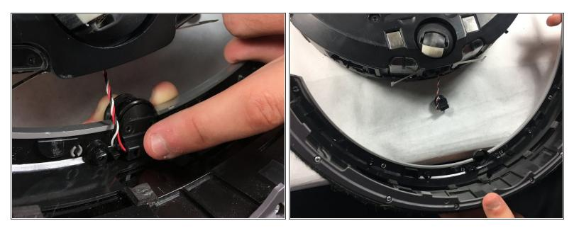
Once the screws are removed, the wire will detach from the bumper and sensor with very light force.
