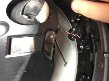
• Using a Phillips #0 screwdriver, remove the two screws.
