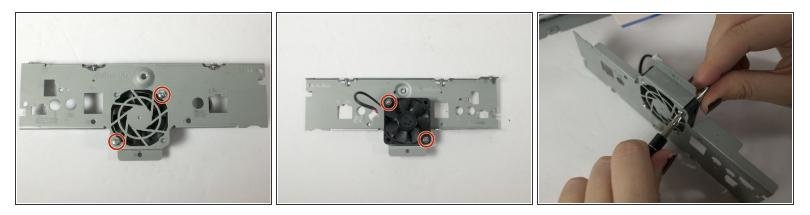
• Remove the two 1-64 x 1/2" machine screws and the retaining nuts that fasten the cooling fan to the rear panel using the Phillips #0 screwdriver and the 5/32" socket.
