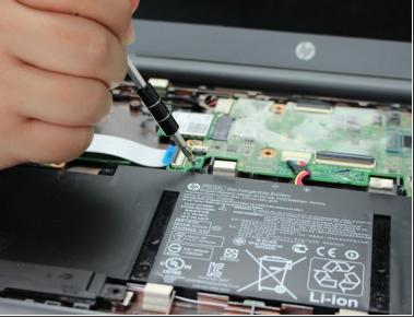
Remove the six 4mm screws holding the battery in place with a Phillips #1 screwdriver.
