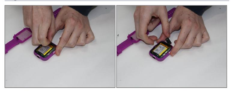
• Carefully remove the speaker from the case without disconnecting it from the motherboard.
