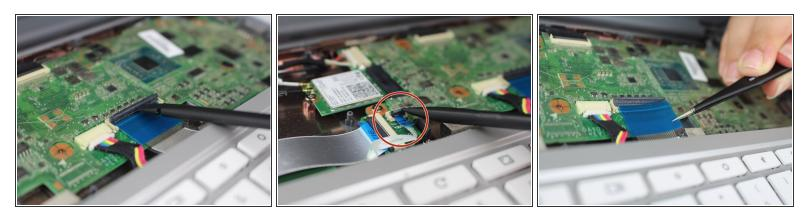
Using the nylon spudger, push the plastic clasps holding the two ribbon wires up to properly disconnect the wires.
