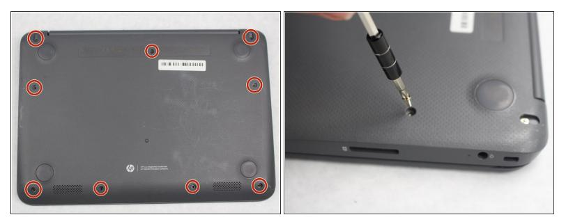
• Turn over your laptop and remove the 9 visible 6mm screws using the Phillips #1 screwdriver.
