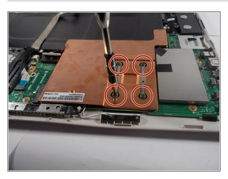
Remove the copper shield by removing the four Phillips screws that hold the shield in place.
