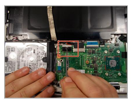
Unplug the battery from the motherboard by pushing the white clip with a metal spudger. You can attempt to use the plastic spudger first, but it may be more difficult.
