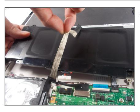
Remove the battery by lifting on the left side, while holding the ribbon cable above it out of the way.
