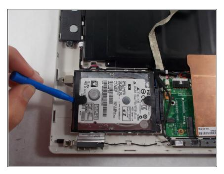
Remove the hard drive using a plastic opening tool.
