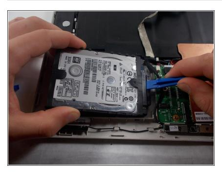
Lift up and unclip the hard drive using the opening tool to pull the plug out.
