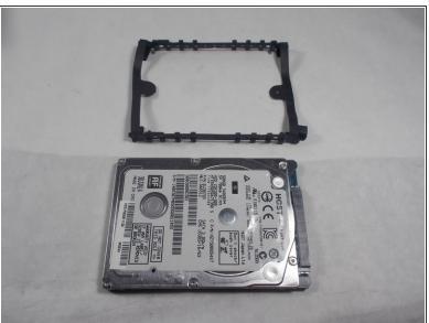
Remove the hard drive from its rubber housing.
