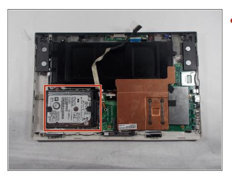
Locate the hard drive in the bottom left of the panel.
