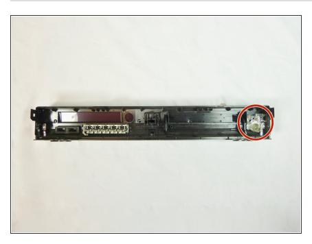
With the inside of the console facing up, the power button will be encased in clear plastic located on the right side of the console.
