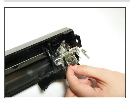
Using your fingers, gently pull out the power button. You can push it from the outside to help loosen it from its hinges. To reassemble your device, follow these instructions in reverse order.
