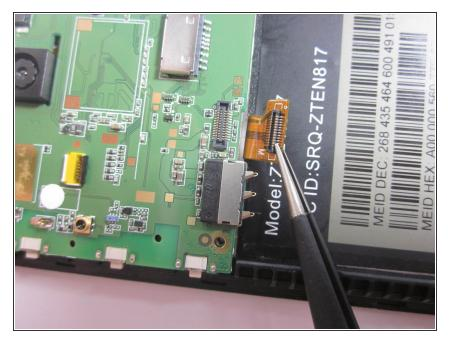
Unplug the flat-top connector by using a pair of tweezers to pry up each side before removing the connector from its socket.
