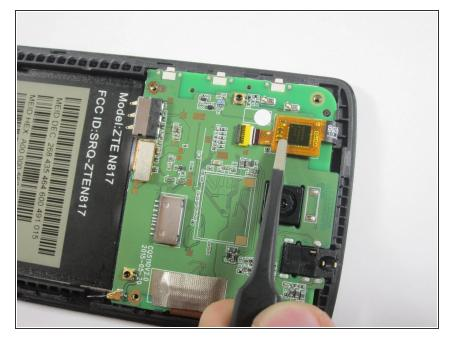
• Use a pair of tweezers to gently disconnect the ribbon cable connector from its socket.
