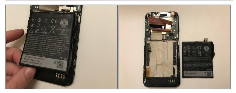
• After prying, simply lift the battery up and out of the device.
