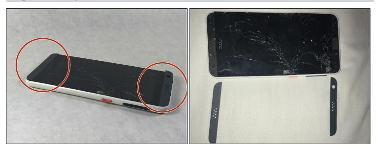
• Use the plastic opening tools to remove the plastic speaker covers that are attached through an adhesive layer.
