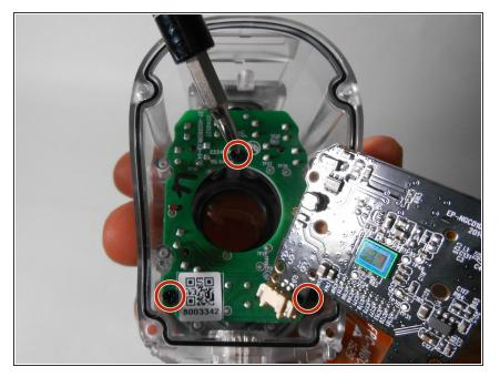
Remove the three 3mm Phillips #000 screws.
