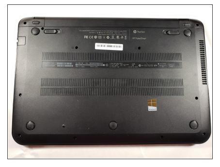
Turn the device upside down and ensure the back of the device is facing you.
