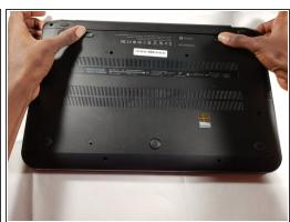
Push both buttons towards one another simultaneously. The battery slightly pops out.
