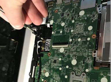
Remove the 5 mm screw using a JIS #1 screwdriver.
