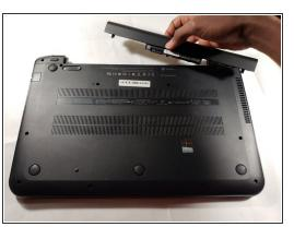
Pull out the battery from the device's battery slot.
