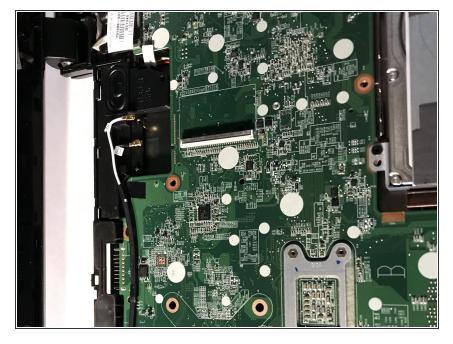
Remove the WLAN card and replace it with a new one.
