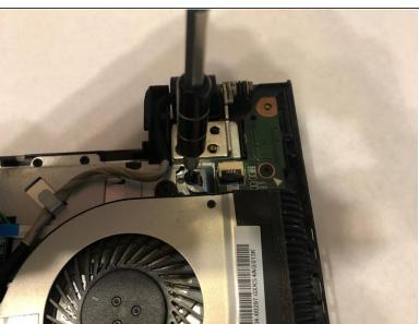
Remove the four M2 x 3mm flat-head screw using a Phillips #000 screwdriver.
