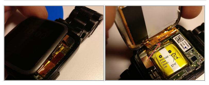
With opening picks we start to open the watch by lifting up the display bottom from left (about seven o'clock) in counterclockwise direction. In the left side there is a flexband that has to be disconnected.
