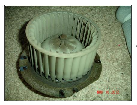
8. Remove the four 5/16" screws that hold the blower motor assembly in the housing and gently pull the motor assembly free from the housing. Note that there is a foam gasket between the motor flange and the duct housing. Also note the orientation of the flat edge of the flange. It faces the outlet of the housing.
