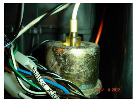
4. Disconnect the white recirc vacuum motor vacuum line from the top of the vacuum motor.
