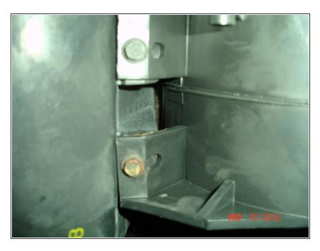
5. Close the glove compartment door and remove the lower two 5/16" screws from under the air inlet duct housing.
