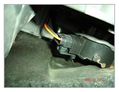
1. Reach back behind the fan motor and disconnect the two pin power plug.
