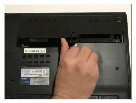
Lift backplate and remove from the case.
