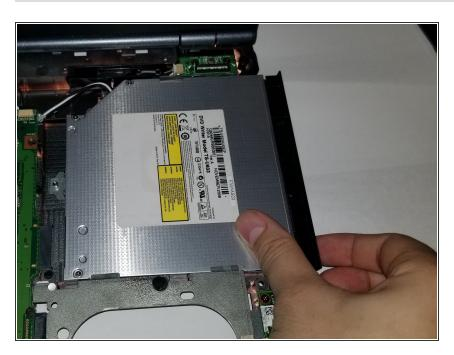
Remove the optical drive by sliding it out from the case.
