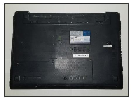
Pull the battery outwards to remove it.
