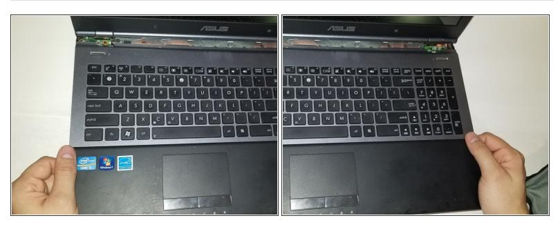
Using both hands, pull the keyboard back and out, fully separating the keyboard from the laptop.
