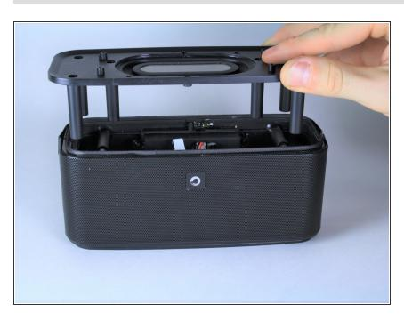
Lift the base-plate off of the enclosure.
