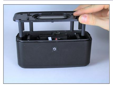
• Lift the base-plate off of the enclosure.
