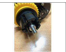
(i) Add wheel spacer on axle which helps to keep tension between bearings
