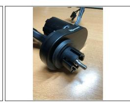
Use 6xM2.5 bolts to attach motor cover to baseplate
