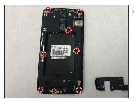
Remove eight 3mm screws using the Phillips #0 screwdriver.
