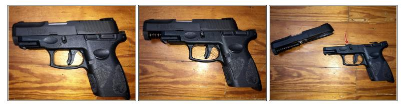
Continue moving the slide forwards until the rear of the slide passes the guides the notches above the disassembly latches(pointed out in the last picture).
