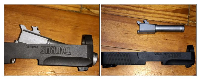
• Lift the barrel out of the slide.
