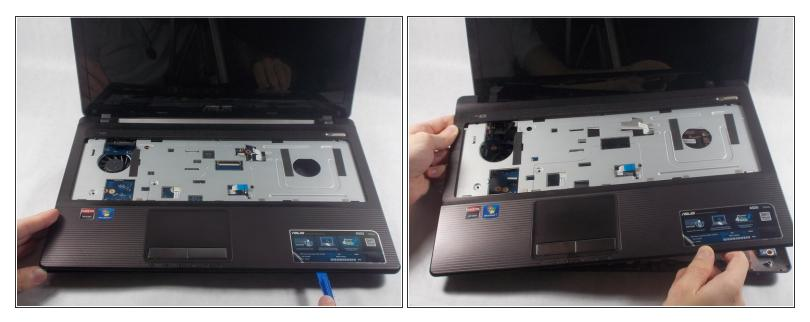
• Separate the front plate of the laptop from the back using the plastic opening tool.
