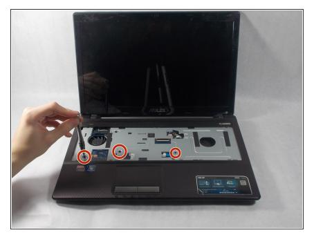
Flip the laptop over again, open it, and unscrew the three 7mm screws using a Phillips #1 screwdriver.
