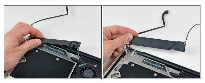
The subwoofer is still connected to the right speaker, so don't completely remove it just yet.
