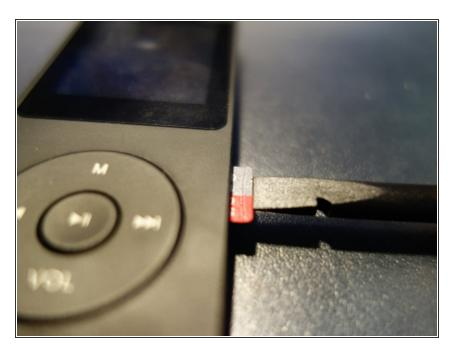
Remove the microSD card, if present. You can use a flat side of a spudger
