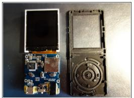
Remove 3 screws with a #00 Philips screwdriver
