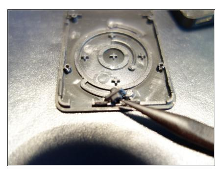
Remove the switch with the shape of a spudger
