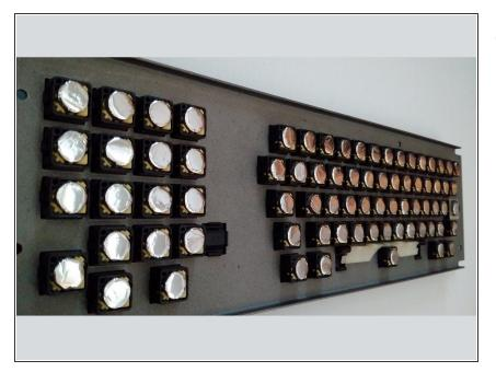
Stick the new foam pad onto the underside of the key mechanism so the sticky side is adhered to the key mechanism and the plastic side of the metal film is oriented toward the circuit board (when Keyboard is reassembled.) Photo credit: deskthority.net
