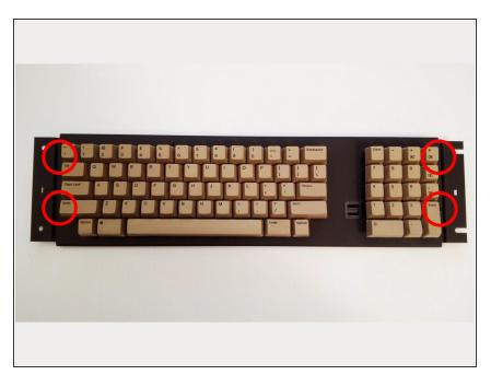
Turn the keyboard around and remove the 4 identified screws.
