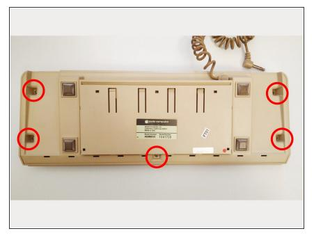
Turn the keyboard over and remove the 5 identified screws. Photo credit: <u>deskthority.net</u>
