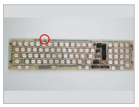
Remove the ground screw. Photo credit: deskthority.net
