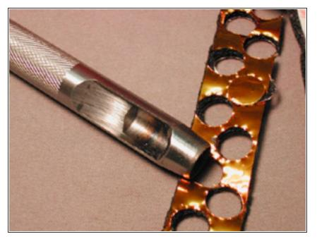
Place foam side down (film side up) on the flat surface. Position the 7/16 punch on the film and hammer firmly with the rubber mallet. Photo credit: lisa.sunder.net
