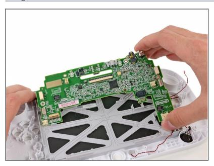
• The GamePad's motherboard is easily displaced from the front panel case.
