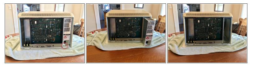
• Release the thumbscrew on the power supply. Pull out the power supply.
