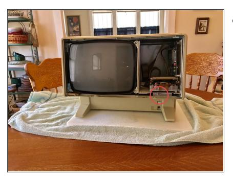
Release the thumbscrew underneath the drive cage and the cage will pull out. Disconnect drive wires while the cage is being removed.
