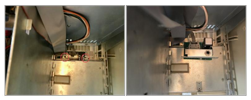
• Release two screws and release the ribbon cable.
