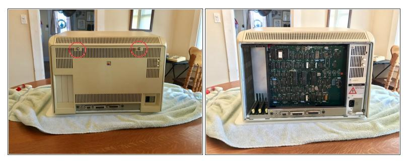
• Twist thumbscrews on the back to release the panel. Pull panel up to remove.
