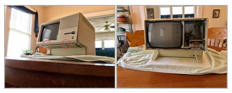
• Press the two tabs underneath to release the panel.
