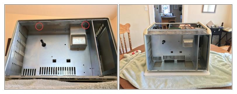
Unscrew two philips screws on the ceiling of where the card cage was.
