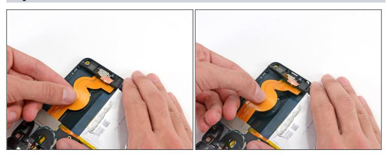
• Grasping the large ribbon cable, gently pull the Lightning connector assembly out of the bottom of the case.
