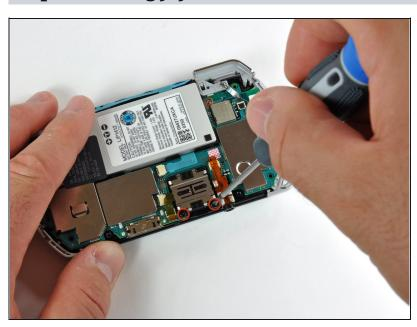
Use a #00 Phillips screwdriver to remove both screws holding the analog joystick in place.
