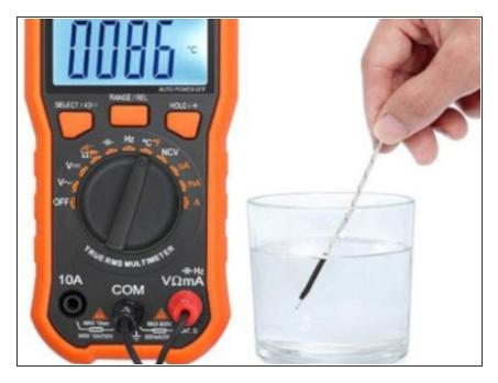
After I replaced the thermostats and tested the machine, I checked the temperature of the boiler with a multimeter and temperature probe. I put the temperature probe under the thermostat clip.
