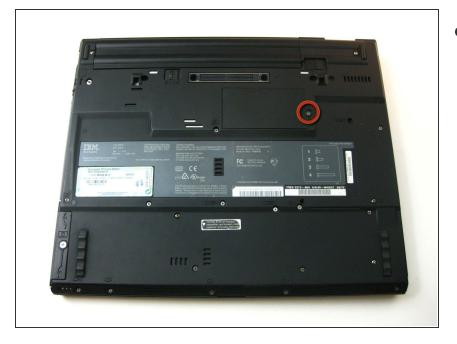
Unscrew the pictured screwed holding the memory cover in place.
