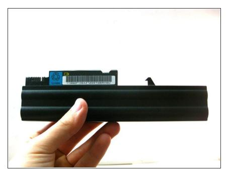
Carefully grab the battery, then pull it straight out, not at an angle.
