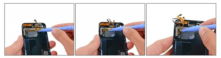
• Slide a plastic opening tool from right to left underneath the horizontal section of the cable, separating it from the adhesive securing it to the rear case.
