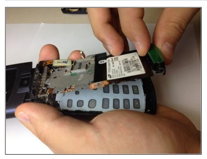
Hold the phone and gently separate the circuit board that holds the dome switches and the front face of the phone, revealing the rubber keyboard.
