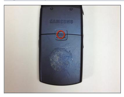
Press on the markings on the cover and pull it down to reveal the battery.
