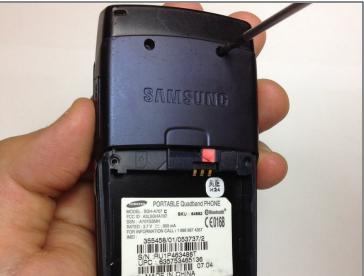
• Unscrew the six screws on the back of the phone using the Phillips #0 screw driver.
