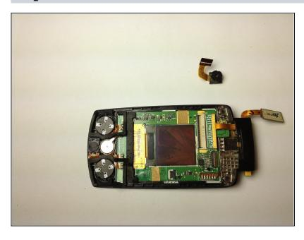
Here is the camera removed from the rest of the phone.
