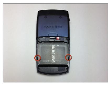
Use your fingers to pull the battery out of its position. You may also flip the phone and the battery will fall out.
