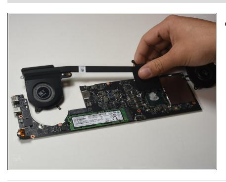
Separate the fans from the motherboard to isolate it for replacement.
