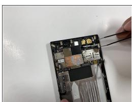
Grab the connectors with the tweezers and gently lift the connectors loose.
