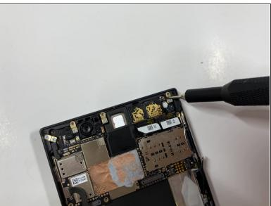
Remove the one 2.5 mm screw with the Phillips #000 screwdriver.
