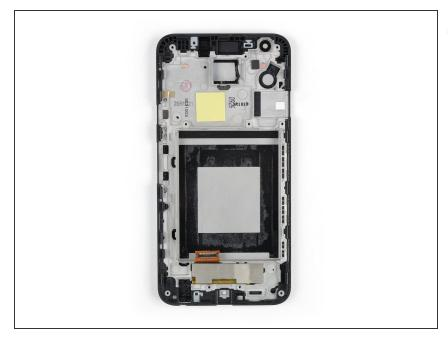
(i) Check your replacement part for any other components that need to be transferred before reassembly.
