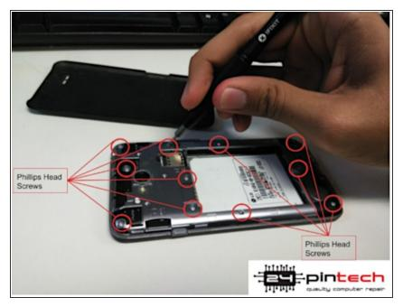
• Remove phillips head screws with a PH000 or similar screw head.
