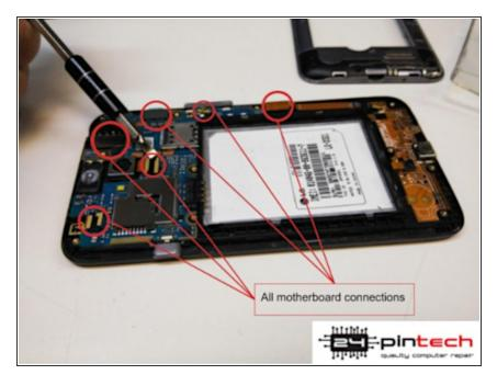
Remove all connections to the motherboard and lift motherboard off of the phone.
