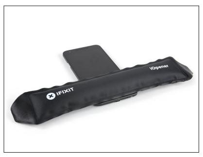
• <u>Use an iOpener</u> on the bottom front of the screen for about 30 seconds to loosen the adhesive beneath the headphone jack.
