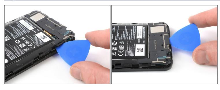
Use the plastic pick to pry open the plastic clips on the long edge of the midframe and on the bottom edge.
