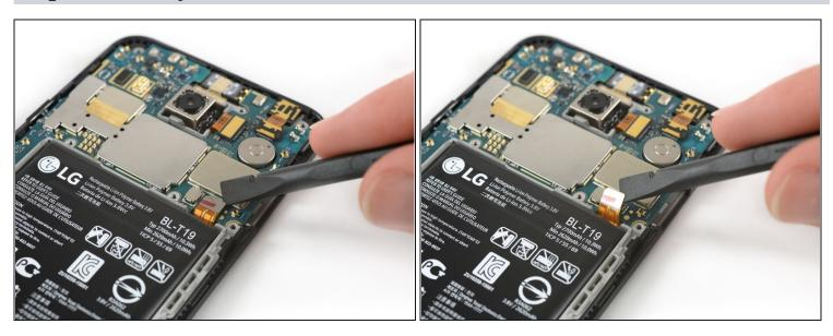
• Use the edge of a spudger to pry up and disconnect the battery flex cable located at the bottom right of the motherboard.
