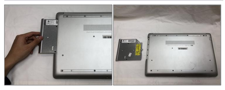
• Slide the optical drive out of the computer.
