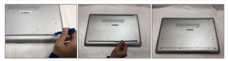
• Using the plastic opening tools, peel back the plastic feet from the underside of the laptop.
