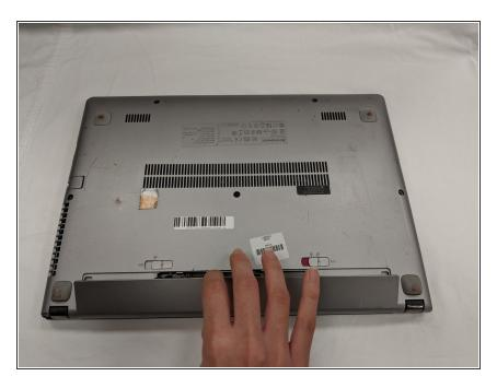
Once both switches are unlocked, the battery will release.
