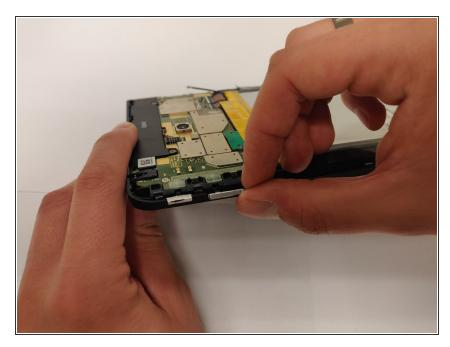
Using your fingers, firmly grasp either the power button or the volume buttons and remove them, releasing the clasps that hold the buttons into place.
