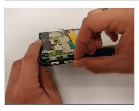
Now, using your fingers replace the buttons that you have removed in the previous step with the new functioning buttons. Enter the button in at an angle and press it into place, clicking it into the open slot. To reassemble your device, follow these instructions in reverse order. To reassemble your device, follow these instructions in reverse order.
