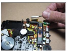
Find Ribbon Cable that connects to the board. Carefully Pry open either side of connector as shown, then remove ribbon cable from board.
