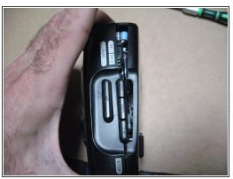
With a small Phillips head, Pry the sides carefully.
