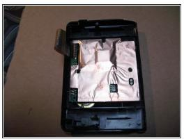
Remove three screws on backside of cassette door. Then remove panel.
