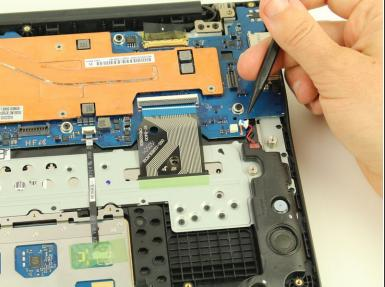
• Use a spudger to disconnect the cables going to the speaker by prying outward to the right.
