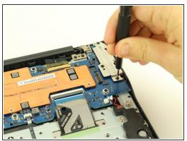
Before you can get to the motherboard, remove the three 4.6mm screws from the port cover using a Phillips #00 screwdriver.
