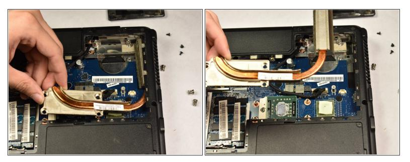
• Pull the heat sink assembly out of the laptop.
