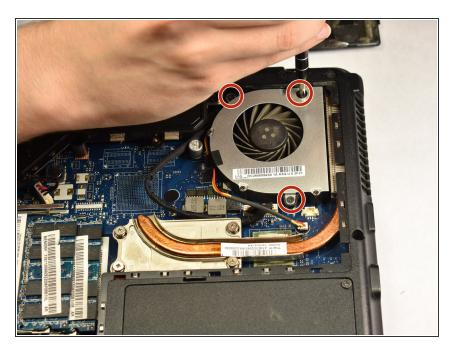
• Unscrew the three 4.6mm screws shown in the picture.
