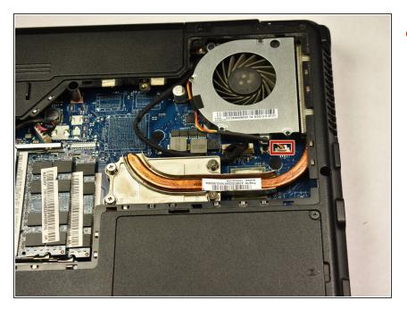
Disconnect the fan from the motherboard by pulling the plug shown in the picture.
