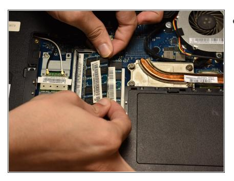
Pull the RAM stick out of its socket.
