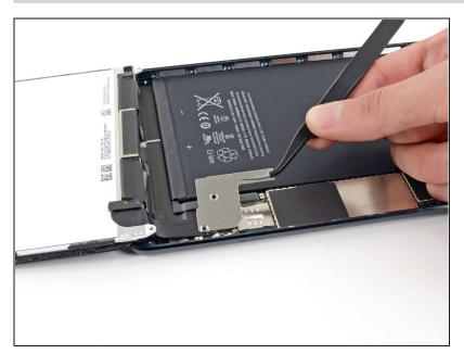
Use a pair of <u>tweezers</u> to grasp and remove the connector shield from the iPad.
