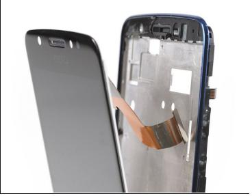
• Carefully thread both display cables through their gaps in the frame.
