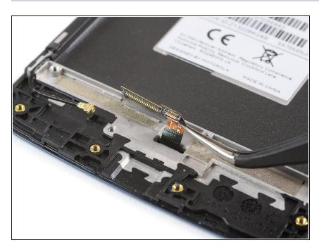
Make sure the fingerprint sensor flex cable does not stick to the frame. If so, peel it loose with a pair of tweezers.
