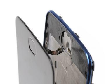
• Carefully thread the fingerprint sensor cable at the bottom through its gap in the frame.
