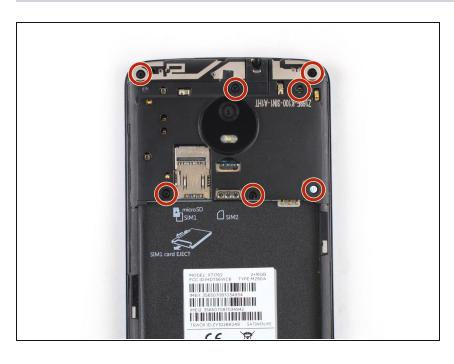
Remove the seven 3.3 mm Phillips #00 screws.
