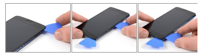
Repeat the previous heating and cutting procedure on the left edge of the phone to cut the remaining adhesive.
