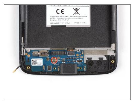
Remove the 2.9 mm long Phillips #00 screw securing the daughterboard.
