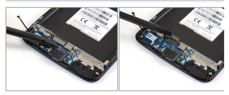
• Use the edge of a spudger to pry up and disconnect the interconnect flex cable.
