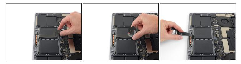
Carefully peel the trackpad cable up off the battery, and push it out of the way.
