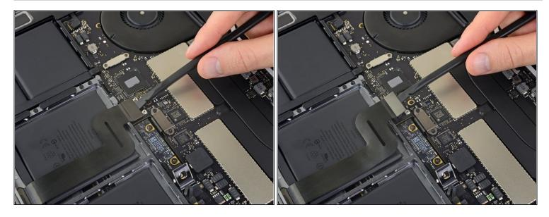
• Use a spudger to disconnect the trackpad cable by prying its connector straight up from the logic board.
