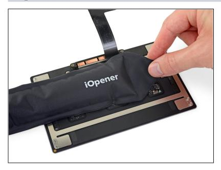
Apply mild heat with an iOpener, hair dryer, or heat gun to soften the adhesive holding the end of the ribbon cable to the trackpad.
