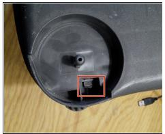
Open the cover of the device and remove the 3 Torx screws. Then pry off the two wheels with a flat screwdriver. Now bend open the clip at the marking with the flat screwdriver.
