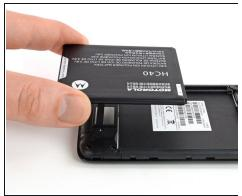
• Use a finger or spudger to lever the battery out of its recess and remove it.
